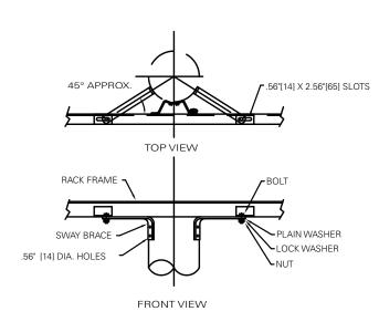
Figure 3. Pole brace installation.
