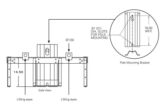
Figure 2. Capacitor rack frame.
