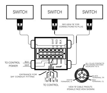
Figure 4. J-Box switched control connections.
