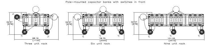
Figure 6. Capacitor rack assemblies 110, 125 and 150 kV BIL with 50, 100, 150, 200, 300, 400, 500, and 600 kvar units
