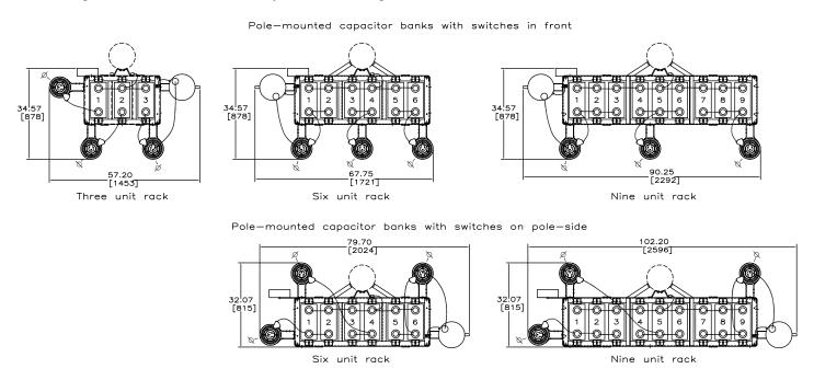
Figure 5. Capacitor rack assemblies 95 kV BIL with 50, 100, 150, 200, 300, 400, 500, or 600 kvar units
